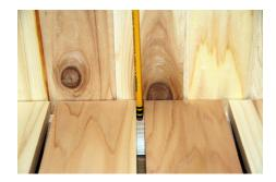
**Step 4:** Position Corner Caps on top of Legs and center on leg. Caps hang over outside of leg roughly 3/4 of an inch. Fasten with **Small** screws using pre-drilled holes. DO NOT OVER TIGHTEN
