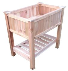
**Step 7:** Position Bottom shelf at desired height (suggest 14" down from upper panel), and slightly in from the edge of the leg. Secure with four (4) **Large** screws in the holes closest to the slats. Use four (4) **Medium** screws in the lower pre-drilled holes.
