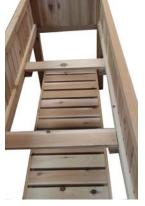
**Step 6:** Place remaining (14) slats inside the planter, resting on the Bottom Supports. NOTE: Evenly space the slats with  $\frac{3}{4}$ " gap. The slats on the ends should be against the legs.
